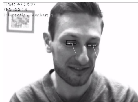
Figure 2. Example output of our eye tracking system. White lines from eyes – eye gaze, black line from top of the nose – head gaze.
